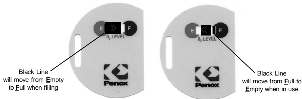
FIGURE 2 - CHECKING THE OXYGEN CONTENTS GAUGE OF THE PORTABLE
